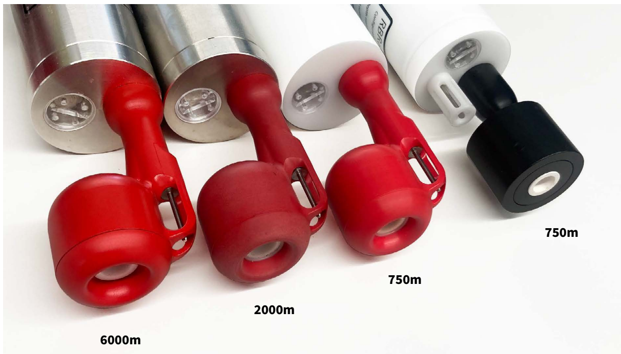
750m-, 2000m-, and 6000m-rated conductivity cells
